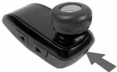
3. While charging, the red LED light will stay on and turn off when charging is complete. You can then unplug the adaptor's connector from the headset and disconnect the adaptor from the electrical outlet.
