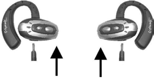
**Note: The ear hook socket port and the power charging port is the same, it means you can either use one port to insert the ear hook, while the other port to charging the battery.**
